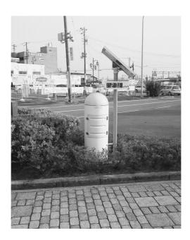
Do you understand what this is? This machine is called a dosimeter. Its purpose, according to the Fukushima prefecture website is to "... monitor the radiation dose rates in areas frequented by children, 2,996 units are installed in the prefecture's schools, childcare centers, parks, etc." Indeed, if you've ever visited the prefecture chances are high you've seen them and perhaps even assumed they had something to do with radiation.
